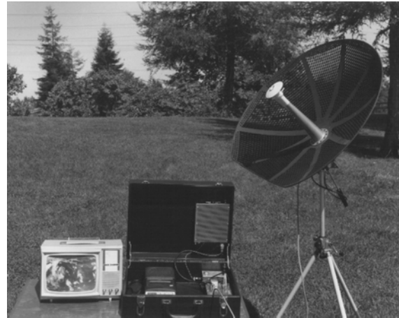
First commercial S-Band WEFAX Receive System, circa 1975
