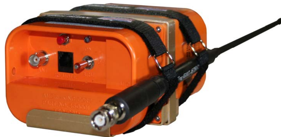
Figure 3: Mounting Tray with Velcro Holder and Portable Antenna for ELT- (AF)(AP)
