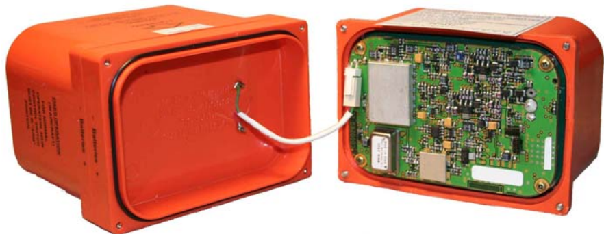
Figure 16: Battery Pack Replacement for ELT Main Unit (Actual View)
