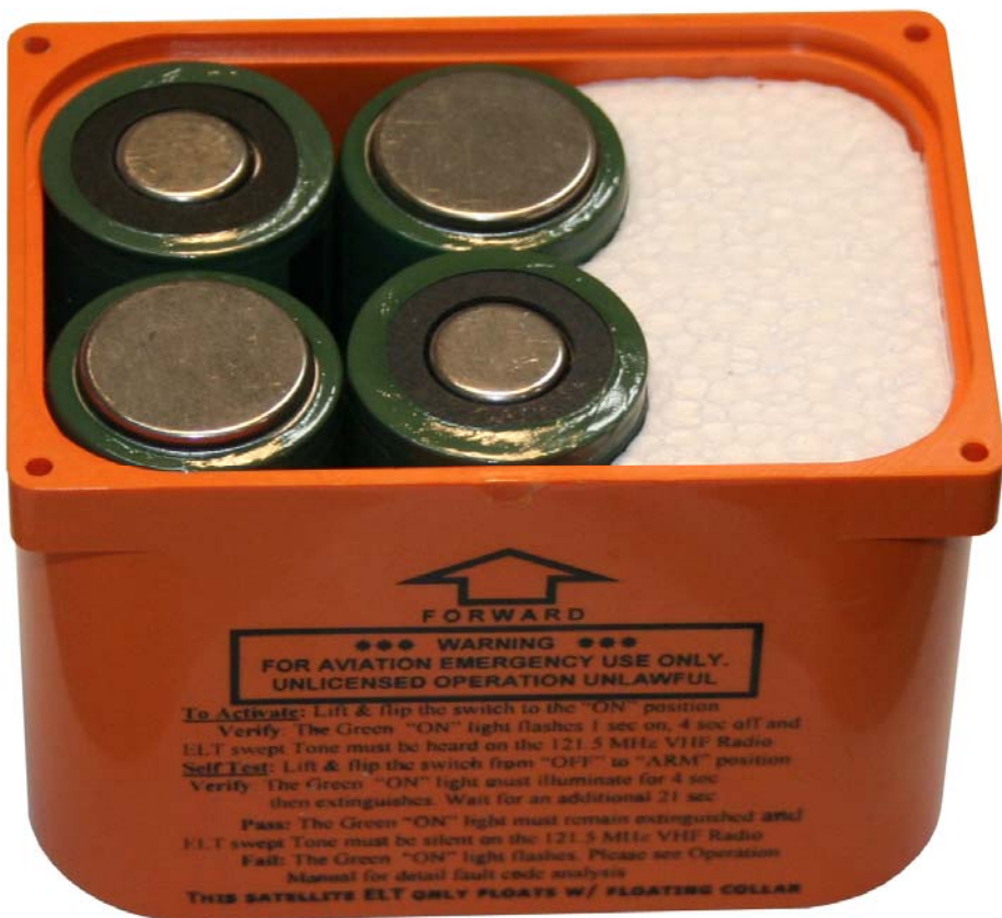
Figure 16.1: Battery Cell Replacement for ELT Main Unit (Actual View)
