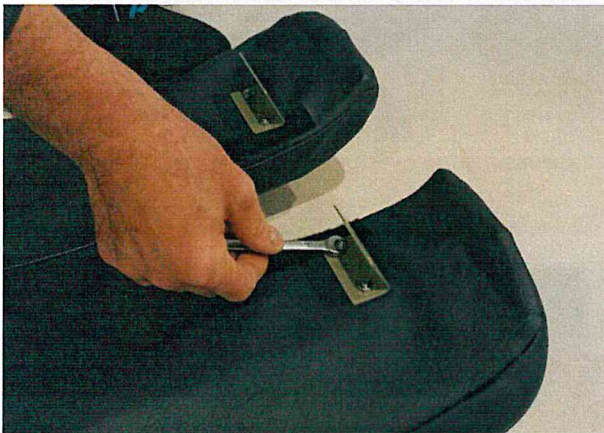
Unscrew the nuts of the original brackets using nut wrench size 8 (5/16")
