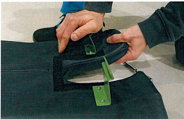
If needed to adjust firmness of the seat attachment in the fuselage, bent slightly the brackets (rearward to reduce attachment force and seat easier insertion into the fuselage), forward in-flight direction to increase seat firmness.
