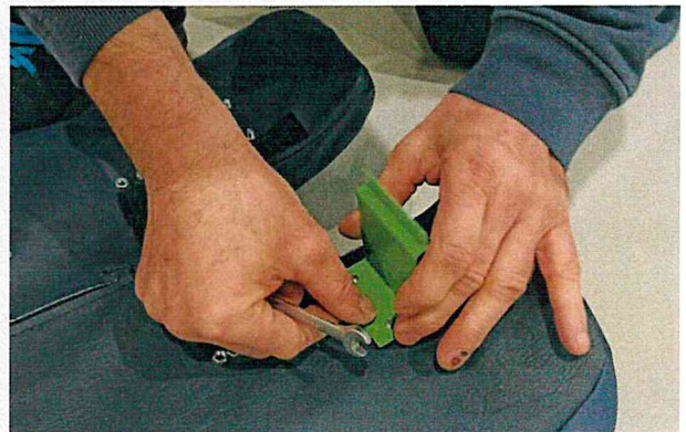
Set the new brackets on the seat.
