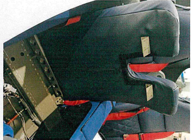
Remove seats from the fuselage
