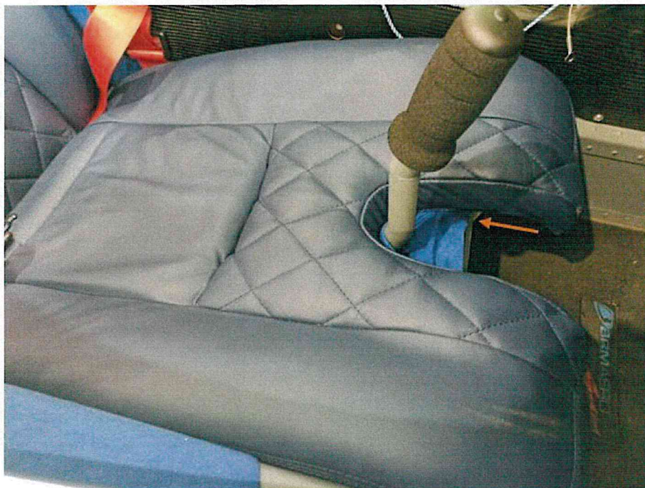
Figure 6 Control stick fully aft limited deflection if the seat jumps up and forward (the console gets in front of the main spar, see arrow).
