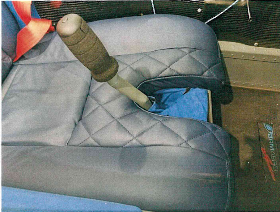
Figure 5 Control stick fully aft deflection if the seat is correctly fitted (brackets behind the main spar).
