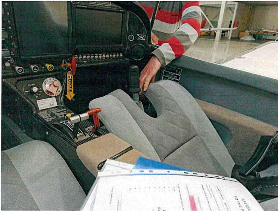
Figure 3 If the seat cushion can be lifted up quite easily, then it is the original design of the seat attachment with straight brackets.
