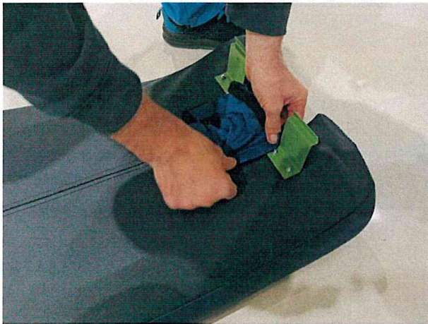
Install the control stick sleeve on the seat velcros.
