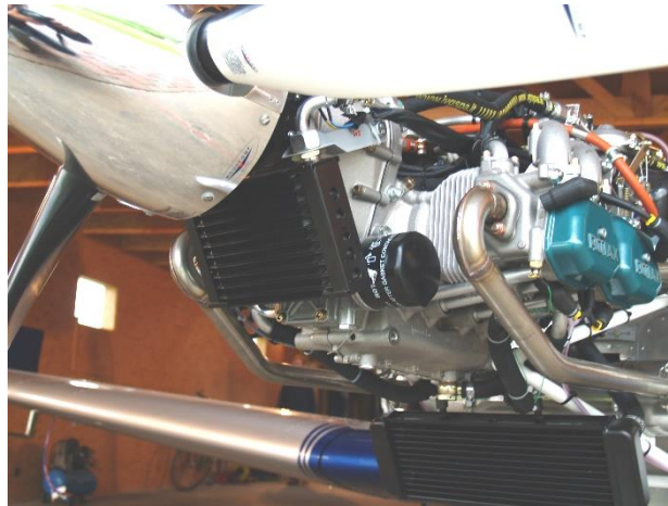
Fig. 10-15 Attachment of the radiator on the engine
