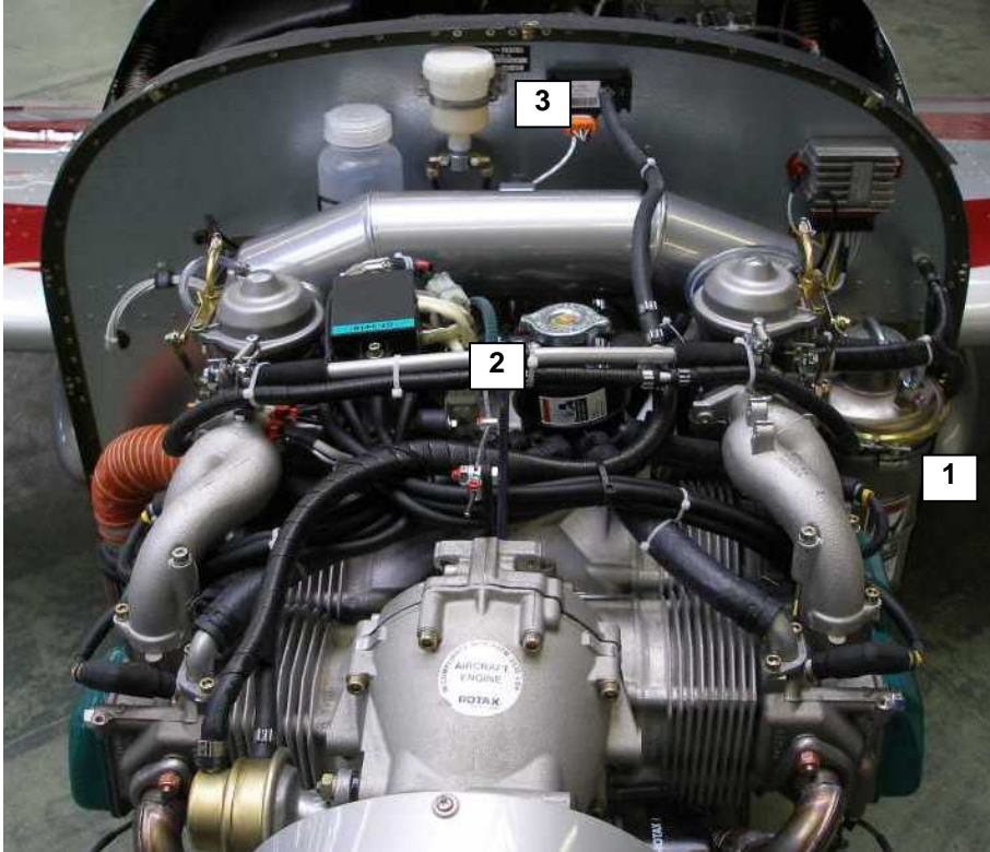
Fig. Filling locations in engine compartment 1- oil tank, 2 - liquid coolant tank 3 – brake fluid central bottle
