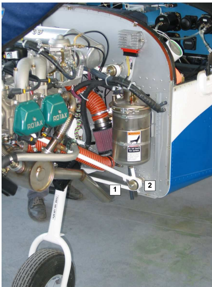
Fig. Engine bed 1- bed, 2 - rubber silentblock
