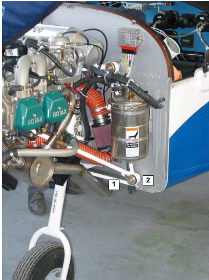
Fig. Engine bed 1- bed, 2 - rubber silentblock
