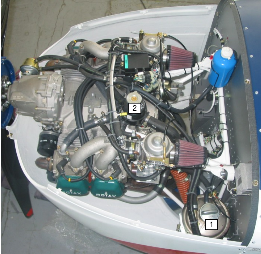
Fig. Filling locations in engine compartment 1- oil tank, 2 - liquid coolant tank
