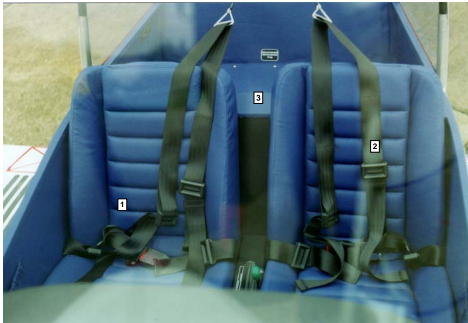
Fig. Cockpit interior 1- seat upholstery, 2 - safety seat belts, 3 - baggage compartment
