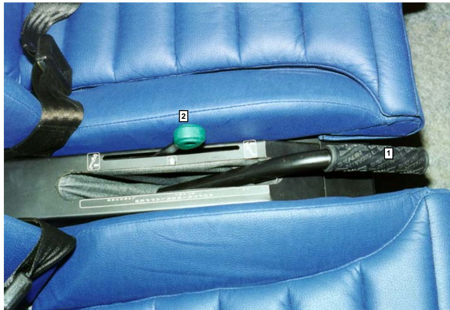
Fig. quadrant between the seats 1- flaps control lever, 2 - elevator trim tab control lever
