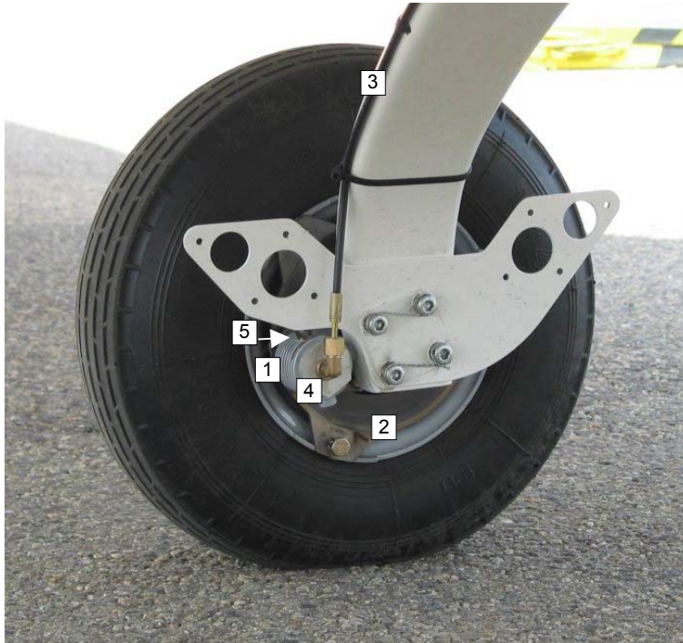
Fig. The brake on the left wheel 1 - brake caliper with the hydraulic cylinder, 2 - brake disc 3 - brake fluid hose, 4 - terminal, 5 - air bleed screw
