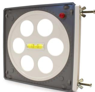
You should be pleased to know that you are using the Warp Drive Professional Protractor which is designed after the high dollar propeller protractors. When used properly this protractor used on Warp Drive propellers, aircraft propellers or airboat propellers, can help you set your propeller blades pitch angle within 1/4 of a degree. It can also be used to check wing surfaces on your aircraft.
