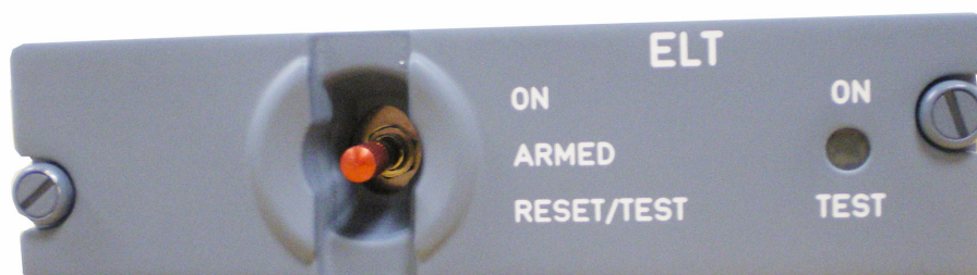
Figure 14: RC800 / 810 Remote Control Panels
