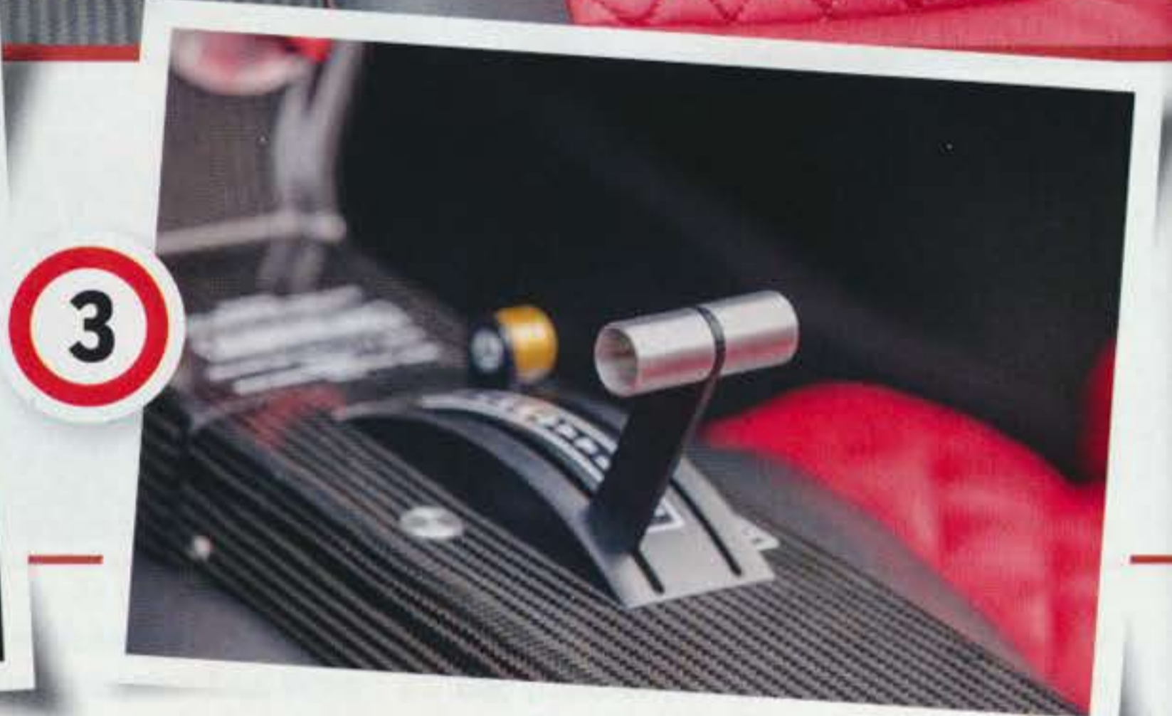
3: nice detail – the proper, T-handle throttle lever and orange-topped choke lever, sharing a central quadrant
