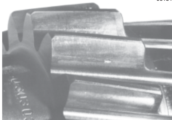
Pitting formation at the foot of spur toothings
