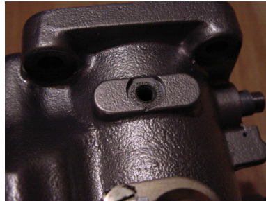
Figure 14-20 Carb Temp Sensor Mounting Location w/Screw Removed
