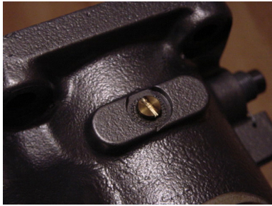
Figure 14-19 Carb Temp Sensor Mounting Location
