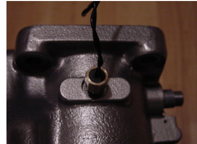
Figure 14-21 Carb Temp Sensor Installed
